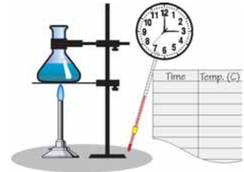
Figure 2.13: An experiment to test the hypothesis that the temperature of water increases proportional to the amount of time you apply the heat.
